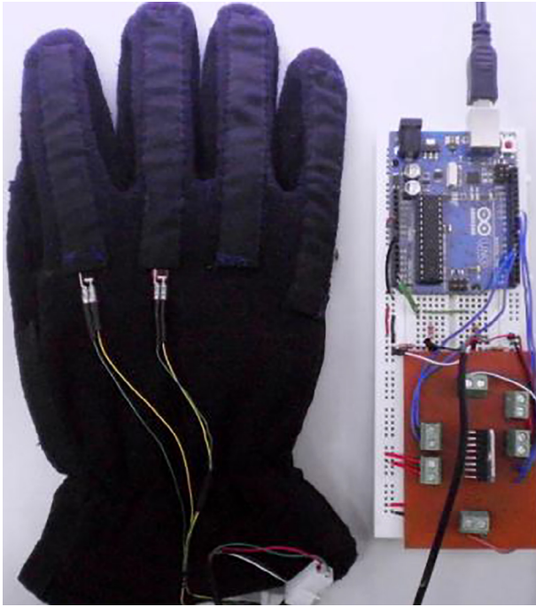
Fig. 1. Contact based electrical resistivity glove shape sensor, known as GloveMAP [8].
