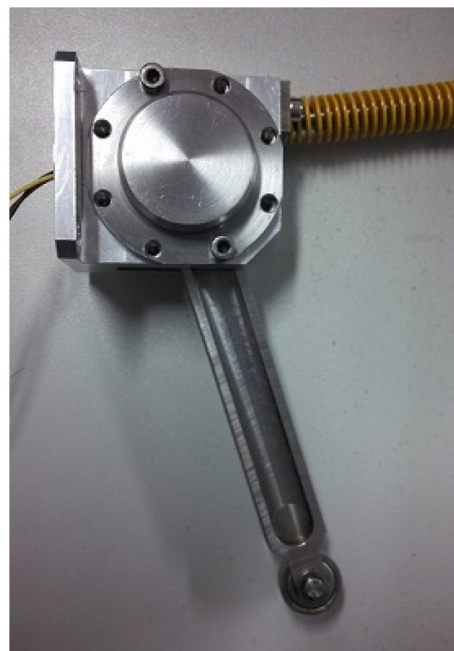
Fig. 2. Schematic diagram and prototype of the wheeled caliper arm.
