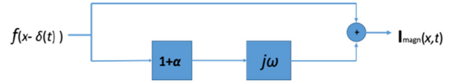
Fig. 1. Temporal filtering applied to each pixel time history. Cut-off frequencies have to be chosen carefully in order to enclose the band of the phenomenon to be analyzed and exclude other frequencies.
