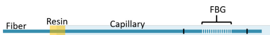
Fig. 1. A schematic representation of the fiber with the FBG, inserted in a glass capillary and fixed on one side with epoxy resin.
