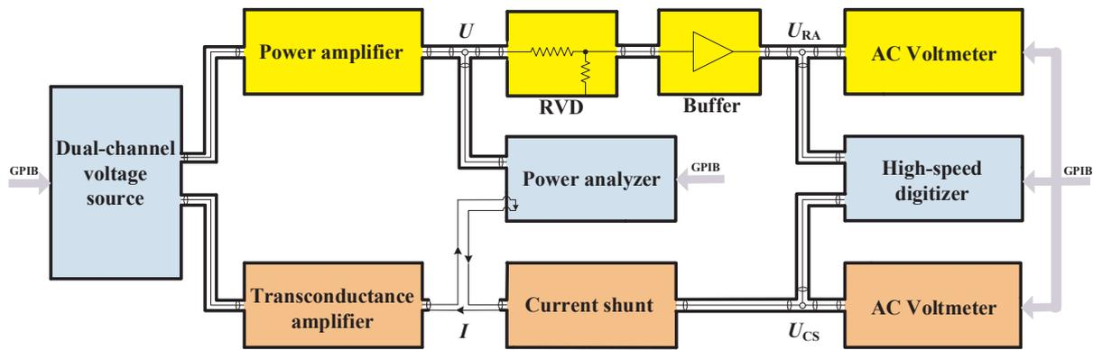
Fig. 1. Diagram of national power standard system.
