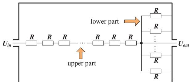
Fig. 2. Basic structure of RVD with serial-parallel connection.
