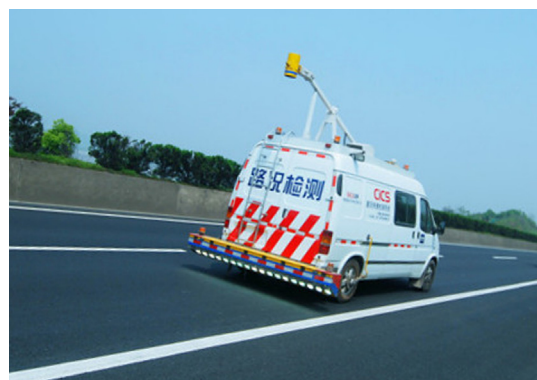
Fig. 2. The vehicle with 13-point laser bar [31].
