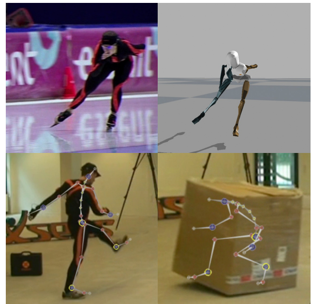
Fig. 1. Examples of inertial motion capture. Upper left: olympic and world champion speed skating Ireen Wüst wearing an inertial motion capture suit with 17 inertial sensors. Upper right: graphical representation of the estimated orientation and position of the body segments. Lower left and right: experiment showing that line of sight visibility is not necessary for inertial motion capture.
