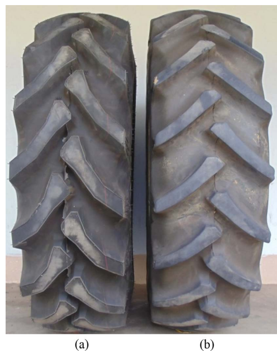
Fig. 1. Test tyres used in the study (a) bias (b) radial.
