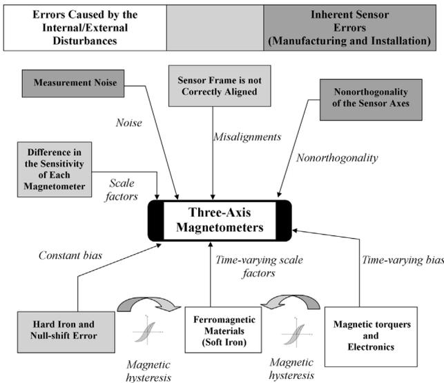
Fig. 1. Magnetometer errors.
