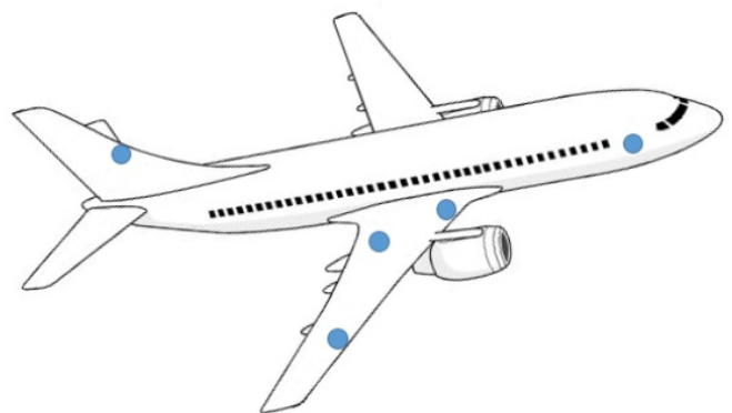
Figure 1: Proposed measurement system, which consists of many pressure sensors distributed on points of interest on the surface of an aircraft [5].
