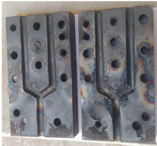
Fig. 1b. Schematic of Y-shape channel actual model.
