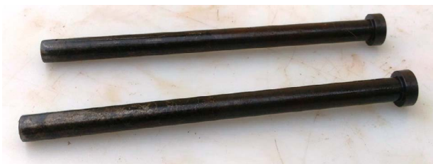
Fig. 1c. Cylindrical punch made of ejector pin.
