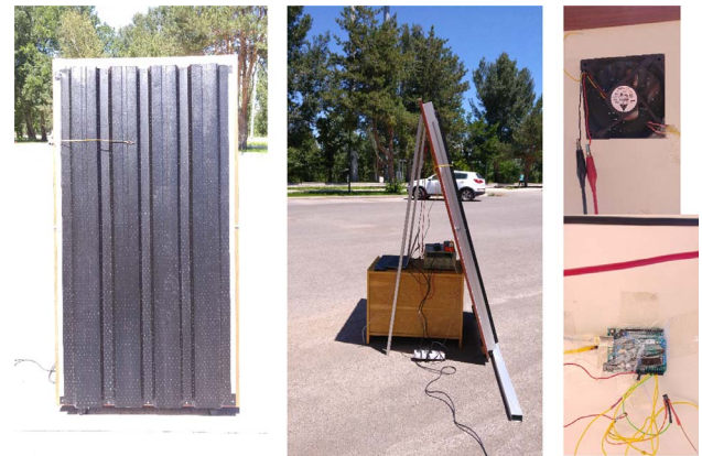
Fig. 2. Experimental setup of the UTC air heating system.
