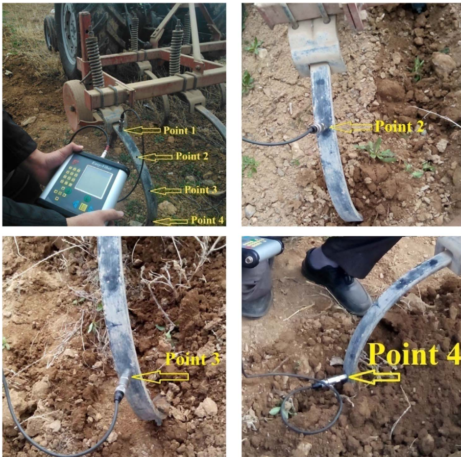
Fig. 1. Photographs of the measurement locations at the chisel plow arm, data acquisition system and accelerometer used in the random vibration test.
