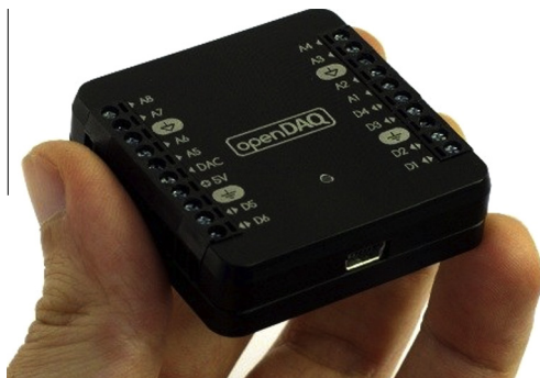
Fig. 2. OpenDAQ top view.
