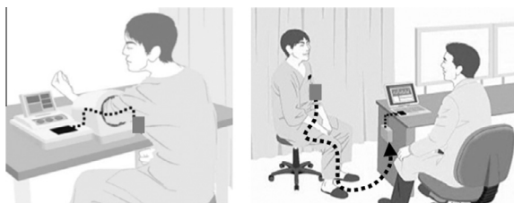
Fig. 2. Sensor data transferred to a doctor's PC by sitting on a chair.
