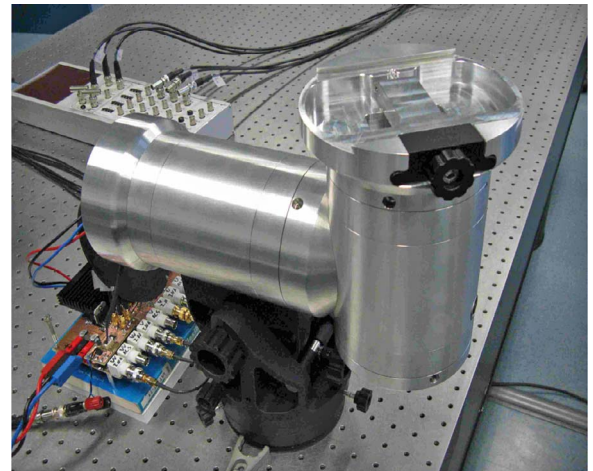
Fig. 1. Laboratory prototype of the two axis rotational servo system with direct-drive PMSMs.
