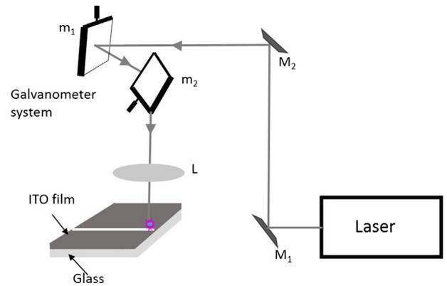
Fig. 1. Schematic of laser set-up for nanograting on glass.
