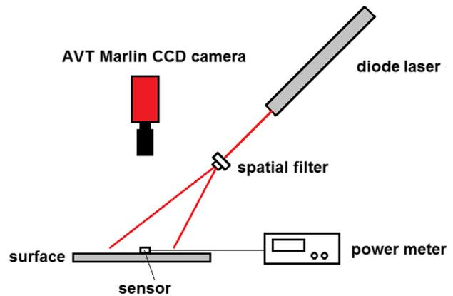
Fig. 1. Experimental configuration used to measure the power of radiation and to acquire speckle patterns using a detector as a power meter of the light in the place of the sample.
