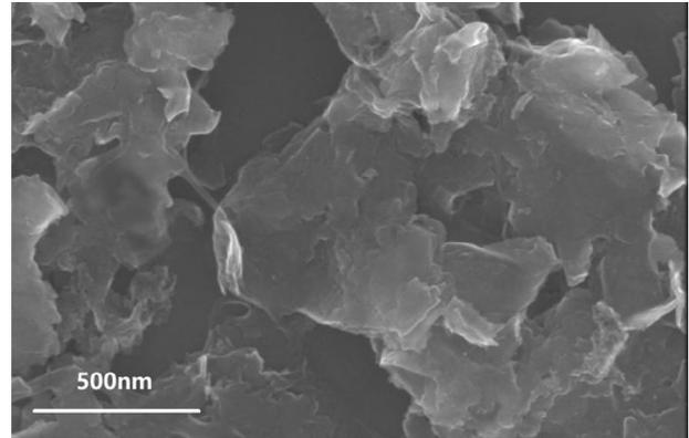
Fig. 2. SEM image of the surface of the MoS<sub>2</sub> absorber.
