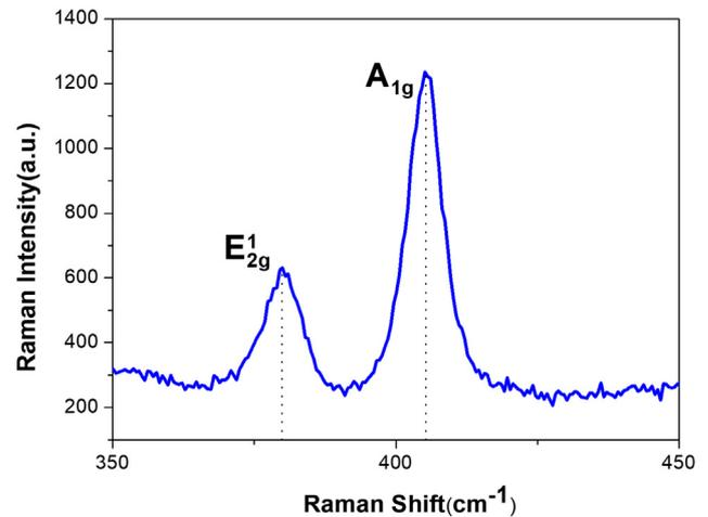
Fig. 3. The Raman spectrum of MoS<sub>2</sub> absorber.
