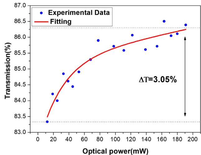
Fig. 4. Nonlinear optical absorption of SA.
