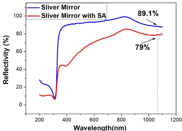
Fig. 1. The reflectance spectrum of the MoS<sub>2</sub> absorber and the silver mirror.
