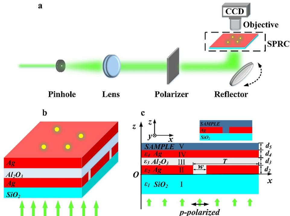
Fig. 1. (a) Schematic of a super-resolution SPRC optical microscopy (SPRC-OM); (b) overall side view of the proposed SPRC structure; (c) section view of the proposed SPRC structure.
