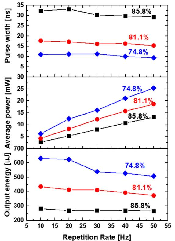
Fig. 3. Q-switched output energy, average power and pulse width of three types of  $\text{V}^{3+}:\text{YAG}$  with various repetition rates.
