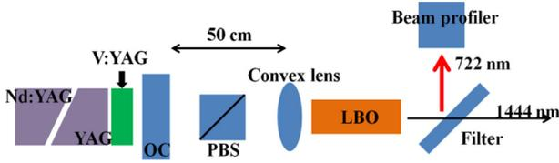
Fig. 1. Experimental setup. PBS : Polarization Beam Splitter.
