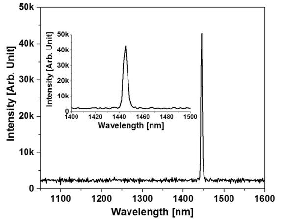
Fig. 2. Output spectrum of 1444 nm laser.
