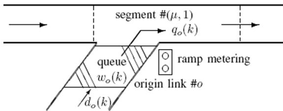
Fig. 1. The origin-link queue model.
