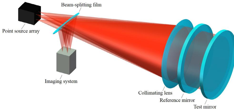
Fig. 1. Optical layout of the proposed interferometer.
