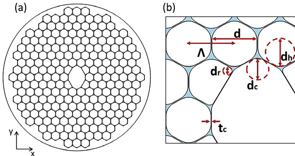
Fig. 1. (a) Cross-section of the 4-cell QEHC-PBGF in numerical simulations; (b) Definition of structural parameters.
