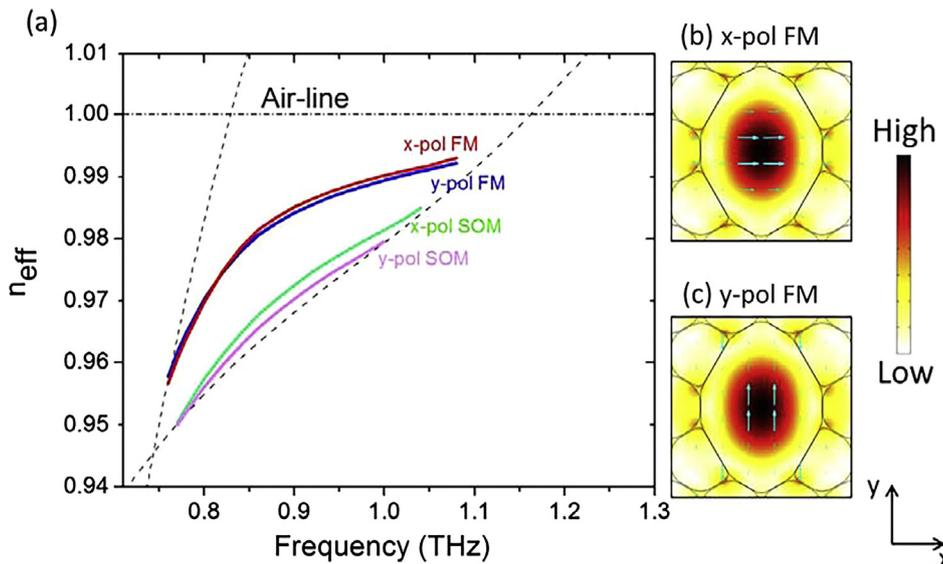
Fig. 2. (a) Photonic bandgap map (dashed curves) and modal  $n_{\text{eff}}$  (solid curves) of 4-cell QEHC-PBGF; Modal fields of (b) x-pol FM and (c) y-pol FM at 0.9 THz.
