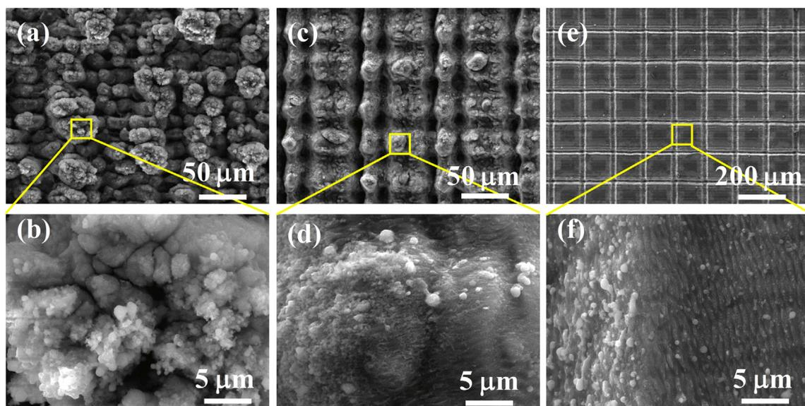
**Fig. 2.** (a–f) Scanning interval dependence of SEM images of the Al surfaces structures by fs laser: (a, b) 10  $\mu\text{m}$ ; (c, d) 50  $\mu\text{m}$ ; (e, f) 200  $\mu\text{m}$ . The laser power is 8 W, and scanning speeds 100 mm/s.
