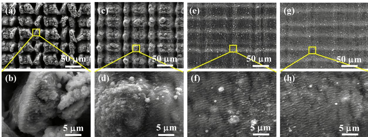
**Fig. 1.** (a–h) SEM images of the Al surfaces' structures by fs laser at different scanning speeds: (a, b) 50 mm/s, (c, d) 100 mm/s, (e, f) 200 mm/s and (g, h) 400 mm/s. The laser power is 8 W and scanning interval 50  $\mu\text{m}$ .
