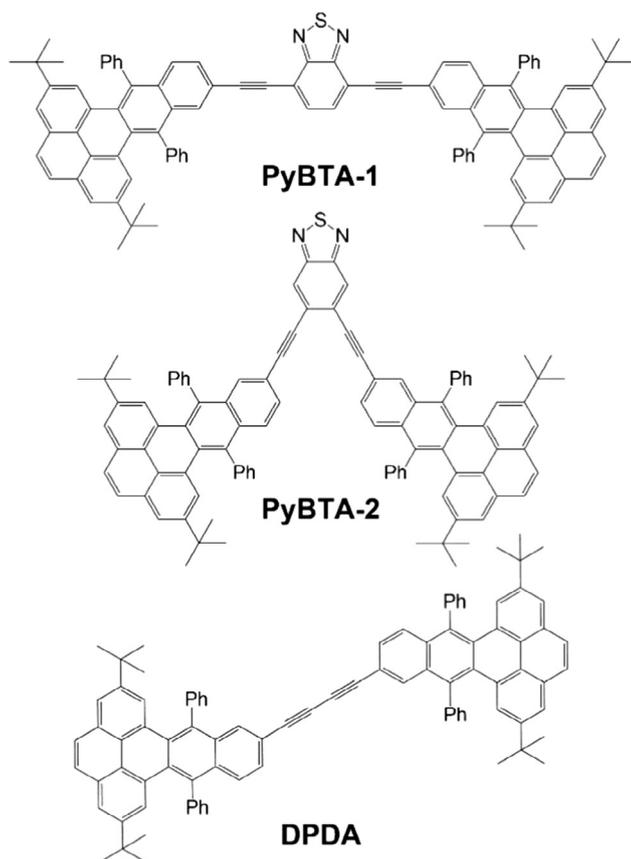
**Scheme 1.** Chemical structures of molecules PyBTA-1, PyBTA-2 and DPDA.
