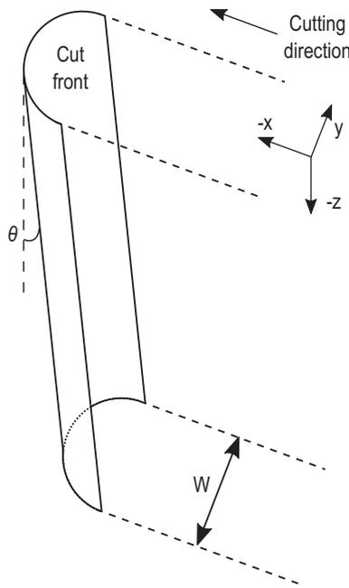
**Fig. 1.** The cutting front described as a half-pipe by Petring et al. [12]. (Kerf width denoted by  $W$  and inclination angle by  $\Theta$ ).
