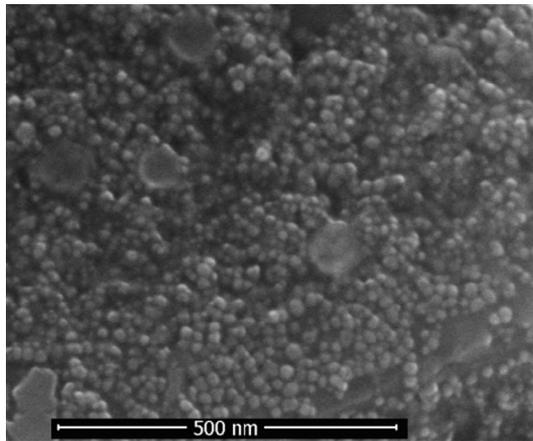
Fig. 1. SEM image of  $\text{Fe}_3\text{O}_4$  nanoparticles.
