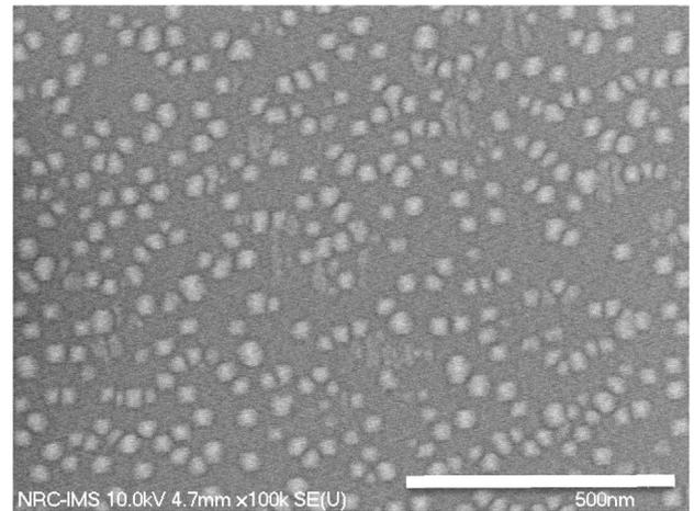
Fig. 2. Scanning electron micrograph of the InAs/InP QD sample surface before any processing.
