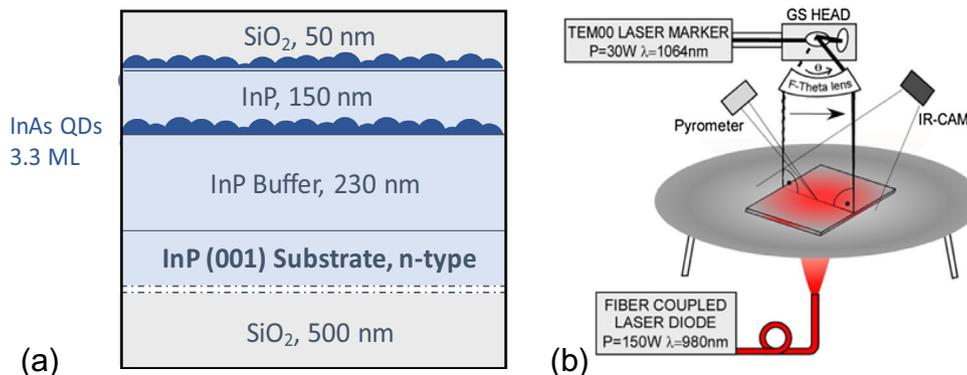
Fig. 1. Cross-section view of the QD microstructure (a) investigated with the ILA technique that makes use of a laser diode (980 nm) and a CW Nd:YAG laser (1064 nm) for selective area annealing of a sample installed on a graphite plate (b).
