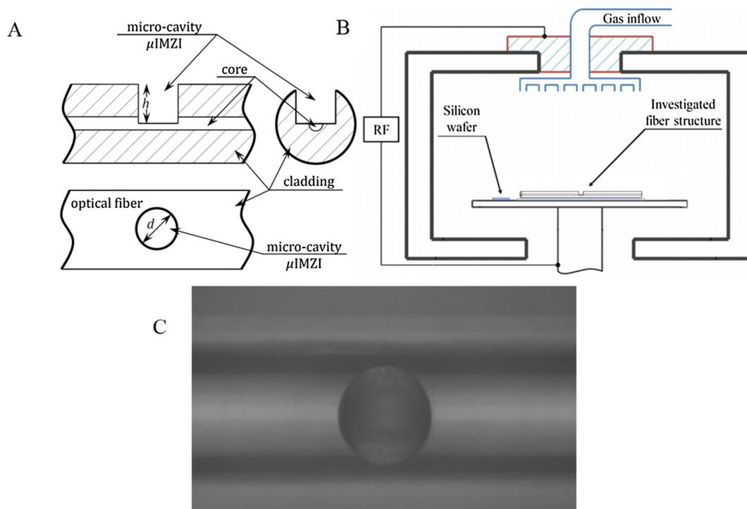
**Fig. 1.** (A) Schematic representation of the  $\mu\text{MZI}$  structure. The diameter of the micro-cavity is indicated by  $d$ , depth by  $h$ . (B) The  $\mu\text{MZI}$  and  $\text{SiO}_2/\text{Si}$  wafer placement in the RIE process chamber. (C) Microscope image of the top view of the microstructure.
