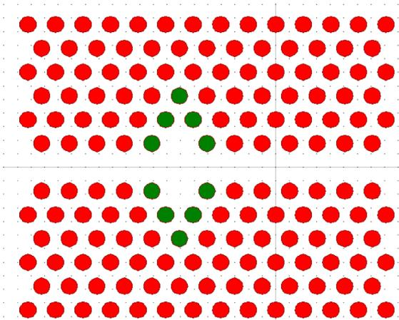
Fig. 2. Schematic of the designed PhC including removed rods and green dots creating the cavity. (For interpretation of the references to colour in this figure legend, the reader is referred to the web version of this article.)
