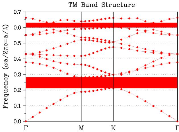
Fig. 1. The simulated band diagram of the designed PhC.
