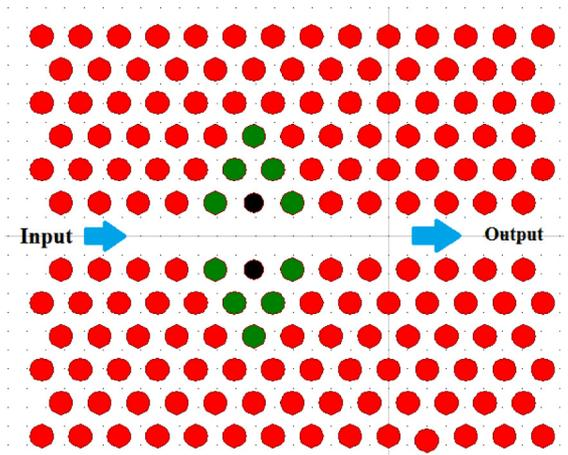
Fig. 5. Schematic of the designed PhC including the located nonlinear Kerr material (black dots) within the cavity.
