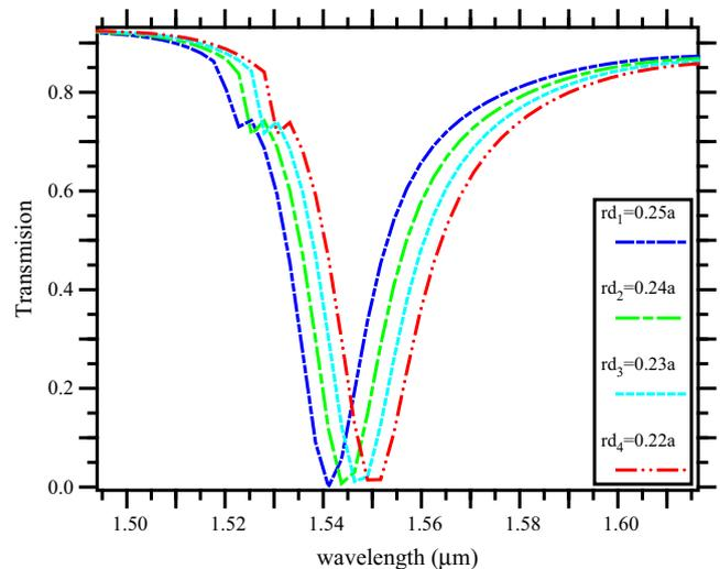
Fig. 6. Simulated transmission vs. wavelength for the PhC with the nonlinear Kerr defects with radii of  $r_{d1} = 0.25a$ ,  $r_{d2} = 0.24a$ ,  $r_{d3} = 0.23a$  and  $r_{d4} = 0.22a$ .
