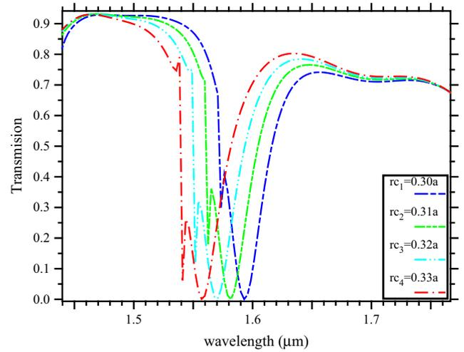
Fig. 4. Simulated transmission vs. wavelength for the PhC with the radii of the rods around the defect of  $r_{c1} = 0.30a$ ,  $r_{c2} = 0.31a$ ,  $r_{c3} = 0.32a$ , and  $r_{c4} = 0.33a$ .
