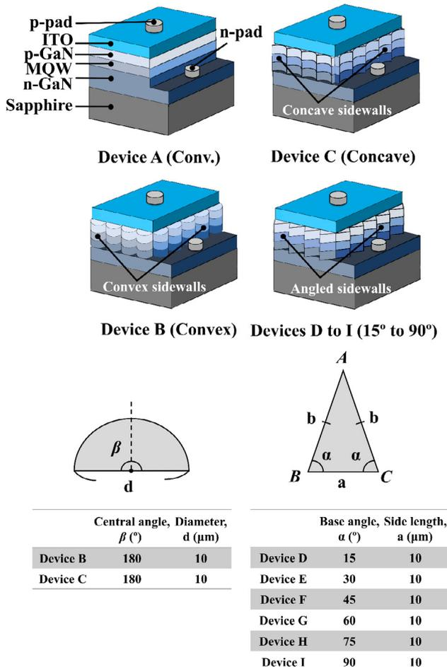
Fig. 1. Schematic cross sections and geometric designs of textured sidewalls of studied devices.
