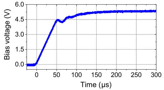
Fig. 2. The voltage on piezo actuator forming the phase shift.
