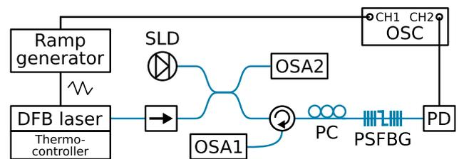
Fig. 3. PSFBG interrogation scheme using single-frequency tunable DFB fiber laser.
