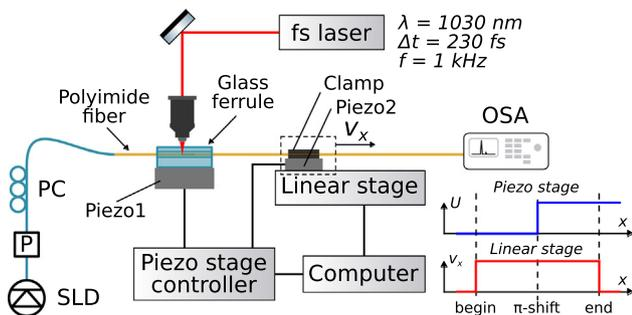
Fig. 1. Experimental setup for PSFBG inscription.
