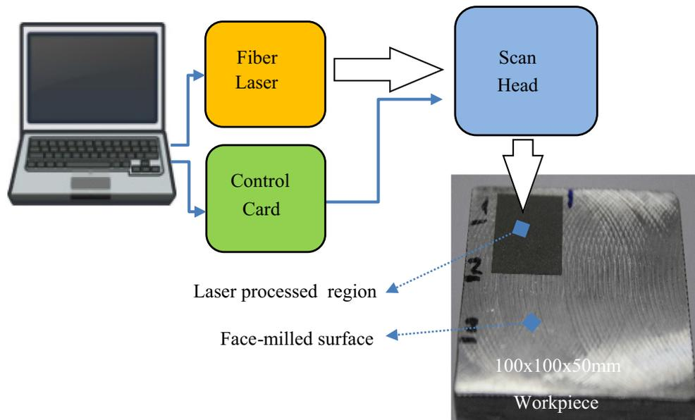
**Fig. 1.** Visual illustration of the experimental set-up, where the scan head is used to move the laser beam on the face-milled aluminum surface and control card is used to control two motors in the scan head.
