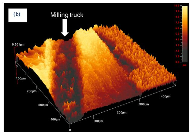
**Fig. 2.** (a) A photograph of milled and laser processed aluminum surface. (b) An optical profilometer picture of the milled surface. The inset pictures in (a) show contact angle measurements of laser processed and un-processed the AA7075 surface.
