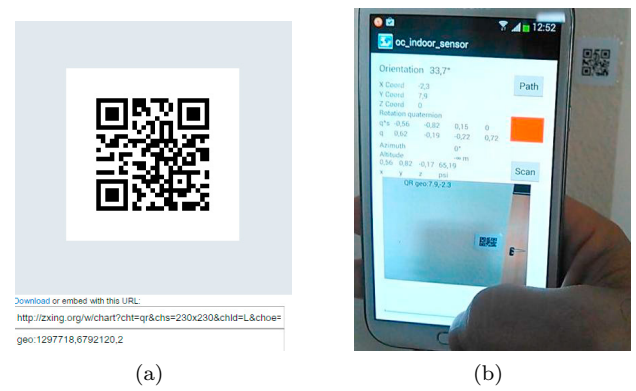
Fig. 3. QR-Code generation (a) and usage (b) for 2.5D coded coordinates of code locations as supplementary navigational aids.
