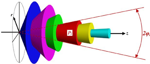
Fig. 3. Idea of conical approximation. Desired 3D light distribution is approximated by finite sum of virtual light cones.
