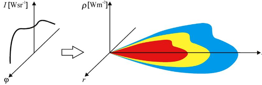
Fig. 2. Angular intensity distribution as a determinant of light distribution in 3D space.
