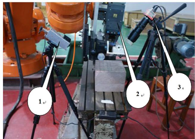
Fig. 1. Laser perforating setup: (1) illumination, (2) laser head and (3) high-speed video.
