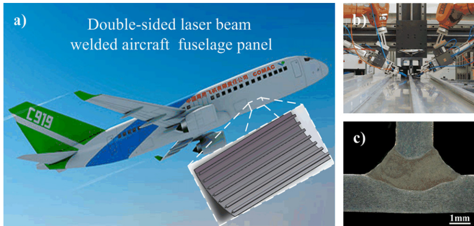
Fig. 1. Double-sided laser beam welded panels in lower fuselage of C919: (a) application location, (b) double-sided laser beam welding system, and (c) cross section of the welded T-joints.
