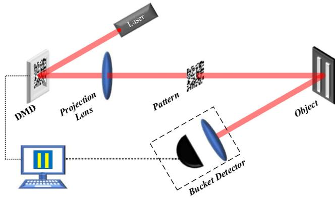
Fig. 1. The schematic diagram of CGI.
