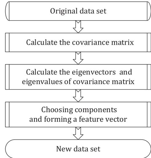
Fig. 2. Flow chart of the principal component analysis process.
