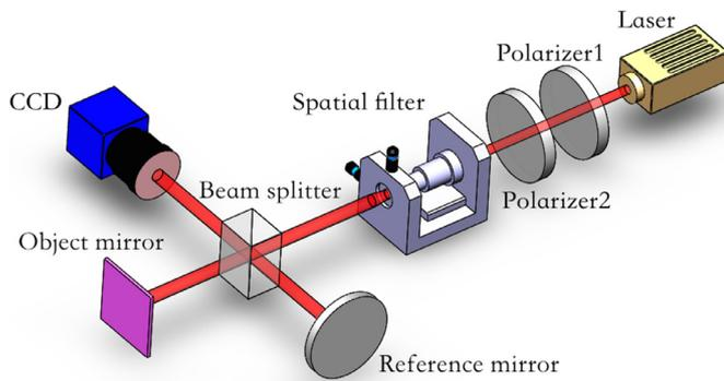
Fig. 1. The structure of the Michelson interferometer.
