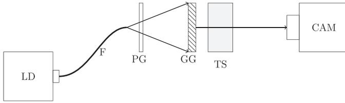
**Fig. 1.** Schematic. LD: Laser Diode, F: Single mode optical fiber, PG: Phase grating, GG: Ground glass, TS: Test Section, CAM: Camera .
