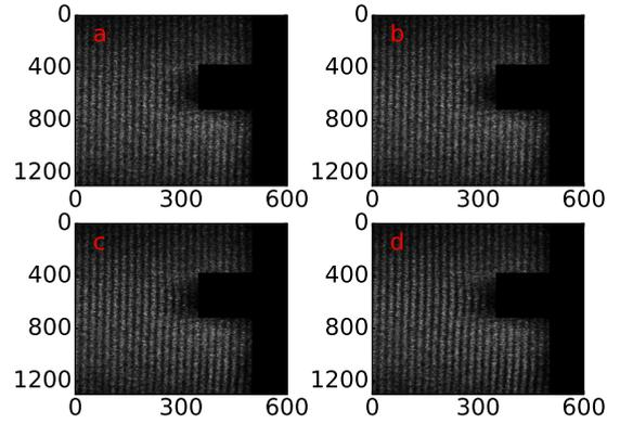
**Fig. 2.** (a) Reference fringe pattern. Fringe patterns obtained for  $\Delta T = 5^\circ\text{C}$ ,  $11^\circ\text{C}$ , and  $18^\circ\text{C}$  in (b–d). The values on the axes represent the number of pixels along the horizontal and vertical directions.
