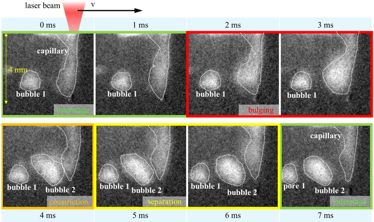
Fig. 1. Series of images out of a high-speed X-ray video showing the formation of a new bubble (bubble 2) during laser beam welding of AlMgSi with  $P = 4 \text{ kW}$ ,  $v = 4 \text{ m/min}$ ,  $d_f = 560 \mu\text{m}$ . The dotted lines highlight the geometries of the voids.
