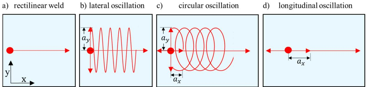
Fig. 2. Applied oscillation patterns and the resulting trajectories of the laser beam path. The amplitudes of the beam oscillation are denoted by  $a_{x,y}$ .
