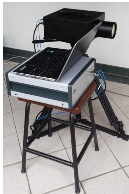
Fig. 2. (a) Schematic layout of optical design of long-distance LDV; (b) prototype of the long-distance laser Doppler vibrometer.
