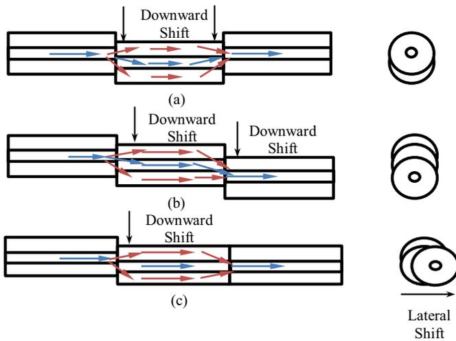
**Fig. 1.** Relative position of the three sections of the U, Z, and L interferometers. It also shows a schematic of the generation of the cladding modes (red) in the middle section and their recombination in the core mode (blue) of the third section. Fig. not to scale. (For interpretation of the references to color in this fig. legend, the reader is referred to the web version of this article.)
