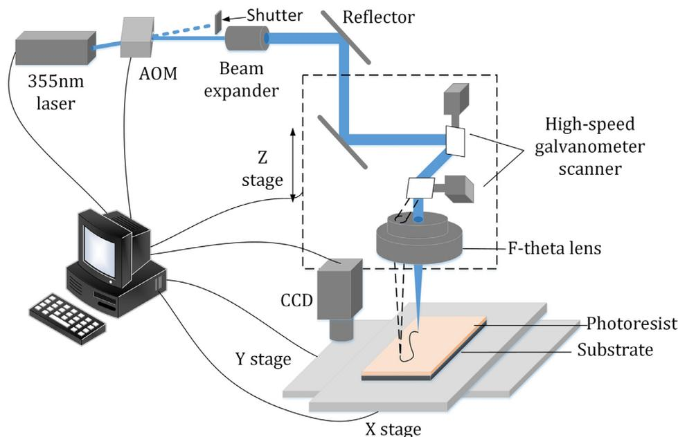
Fig. 1. Schematic diagram of focused laser lithographic system.
