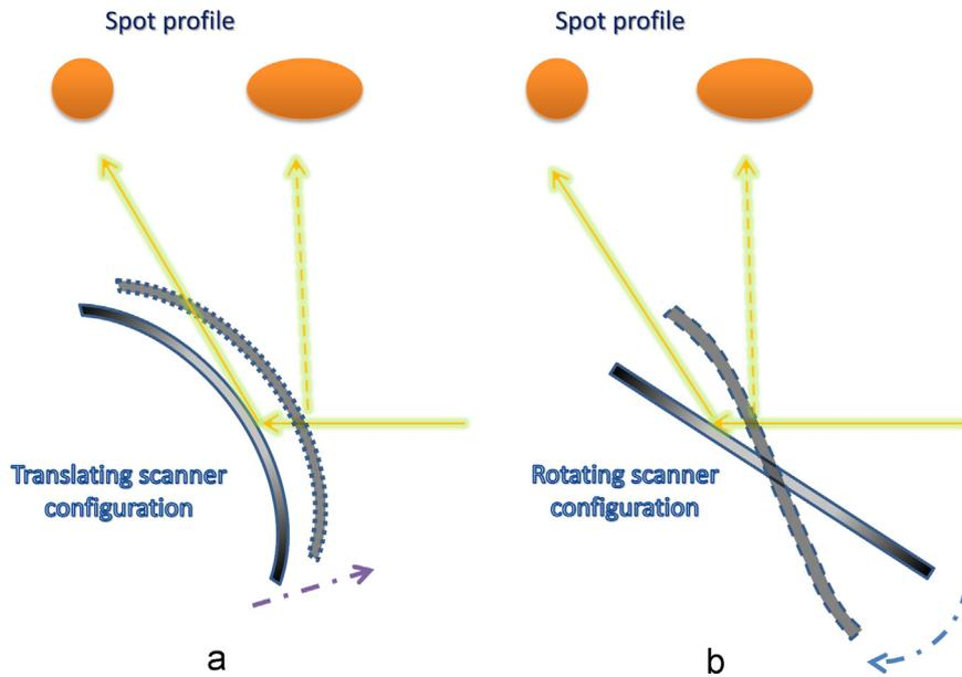
Fig. 1. Beam spot size variation as a result of using linearly moving curved micromirrors in (a), and rotating flat micromirrors in (b) with dynamic deformation.
