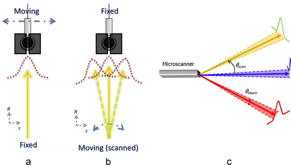
Fig. 2. (a) Conventional beam characterization method for a static beam by the linear motion of a detector covered by a slit. (b) Proposed method for characterizing a scanned beam as a function of the scanning angle utilizing a fixed detection system and an angularly scanned beam. A Gaussian profile for the beam intensity is given in the figure for illustration. (c) An output beam from a microscanner at a given radial distance has a divergence and a scanning angle.
