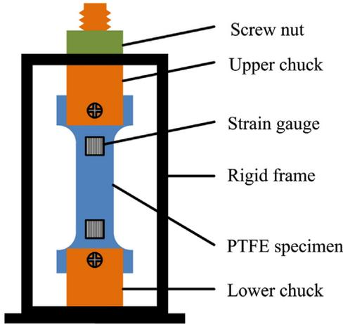
Fig. 2. Mechanical loading device.
