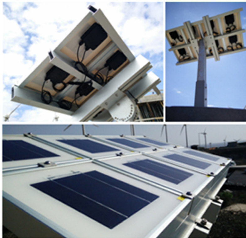
Fig. 1. Outdoor setup: tilting head (up-left), exchangeable pillar (up-right) and modules attached with clamps (down).
