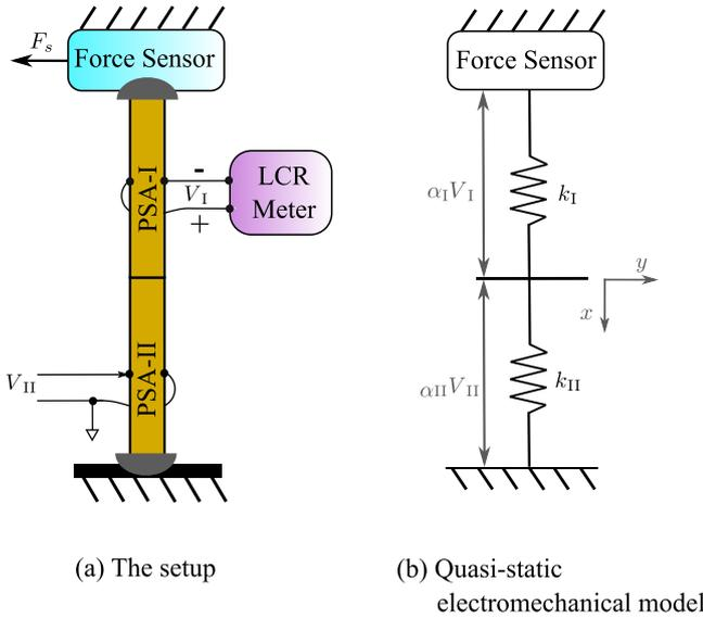
**Fig. 1.** The setup used for studying the effect of external loads on the impedance of a piezoelectric actuator.
