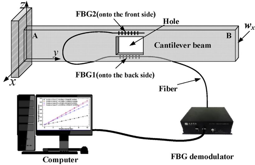
Fig. 1. Schematic diagram of the system for displacement measurement.
